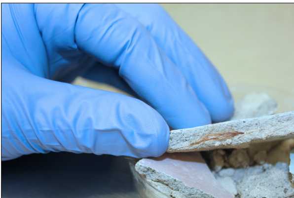
Asbestos fibers in building materials
