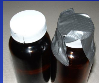
Cracked bottle or cap
